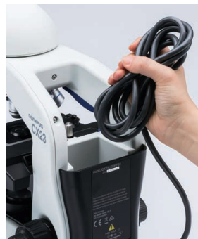
Cable storage compartment
